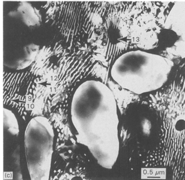
Figure 33 STEM micrograph of the laser-clad Ni-Hf alloy showing the X phase and eutectic phase. Inset is a schematic diagram showing the positions of the probe from where microanalysis was performed.
