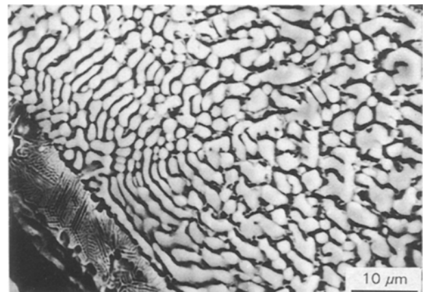
Figure 38 Scanning electron micrograph of the laser-clad Fe-Cr-W-C alloy showing uniform distribution of tungsten carbide precipitate.
